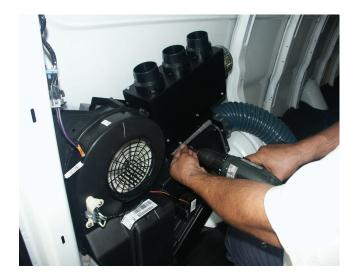
There are two (2) ducts on the factory HVAC unit. One at rear is for air conditioning and one forward is for heat. The 4" blue hose connects heat into the new plenum.
